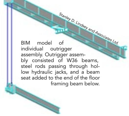
BIM model of individual outrigger assembly. Outrigger assembly consisted of W36 beams, steel rods passing through hollow hydraulic jacks, and a beam seat added to the end of the floor framing beam below.
